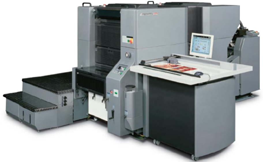
A Creo (Canadian company) DI (direct imaging) offset press, developed to make press operation possible by non-tradespeople, to speed up the whole printing process, and reduce the viable run length to somewhere around 250-300.
